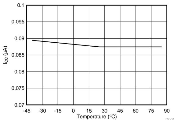
Figure 1. I<sub>CC</sub> Variation With Temperature
