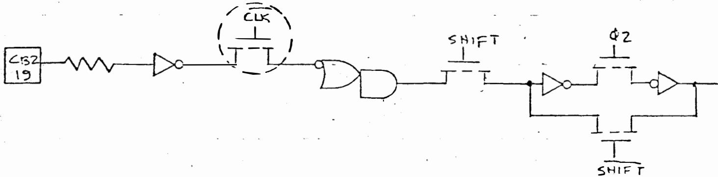
(3) PROBLEM: WHEN SHIFTING IN OR OUT UNDER CONTROL OF T2, THE TIME FROM A SR READ OR WRITE TO THE FALLING EDGE OF THE FIRST CLOCK PULSE DEPENDS UPON THE INITIAL CONTENT OF T2.
