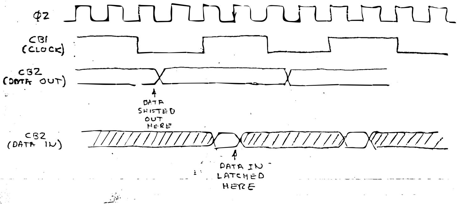
THE TIMING SHOULD BE MODIFIED SO THAT DATA IS REFERENCED TO THE CLOCK EDGE AS SHOWN BELOW!
