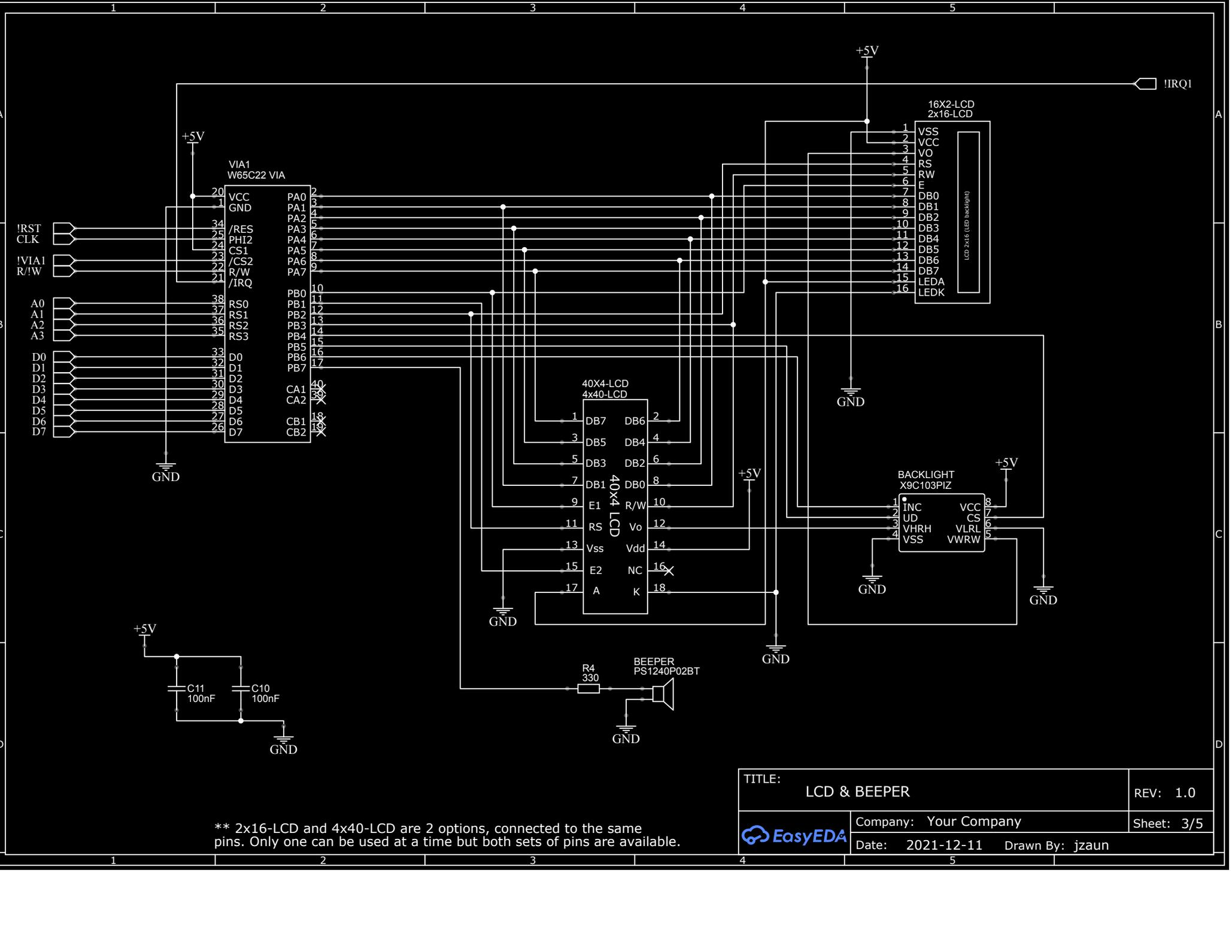
\*\* 2x16-LCD and 4x40-LCD are 2 options, connected to the same pins. Only one can be used at a time but both sets of pins are available.
