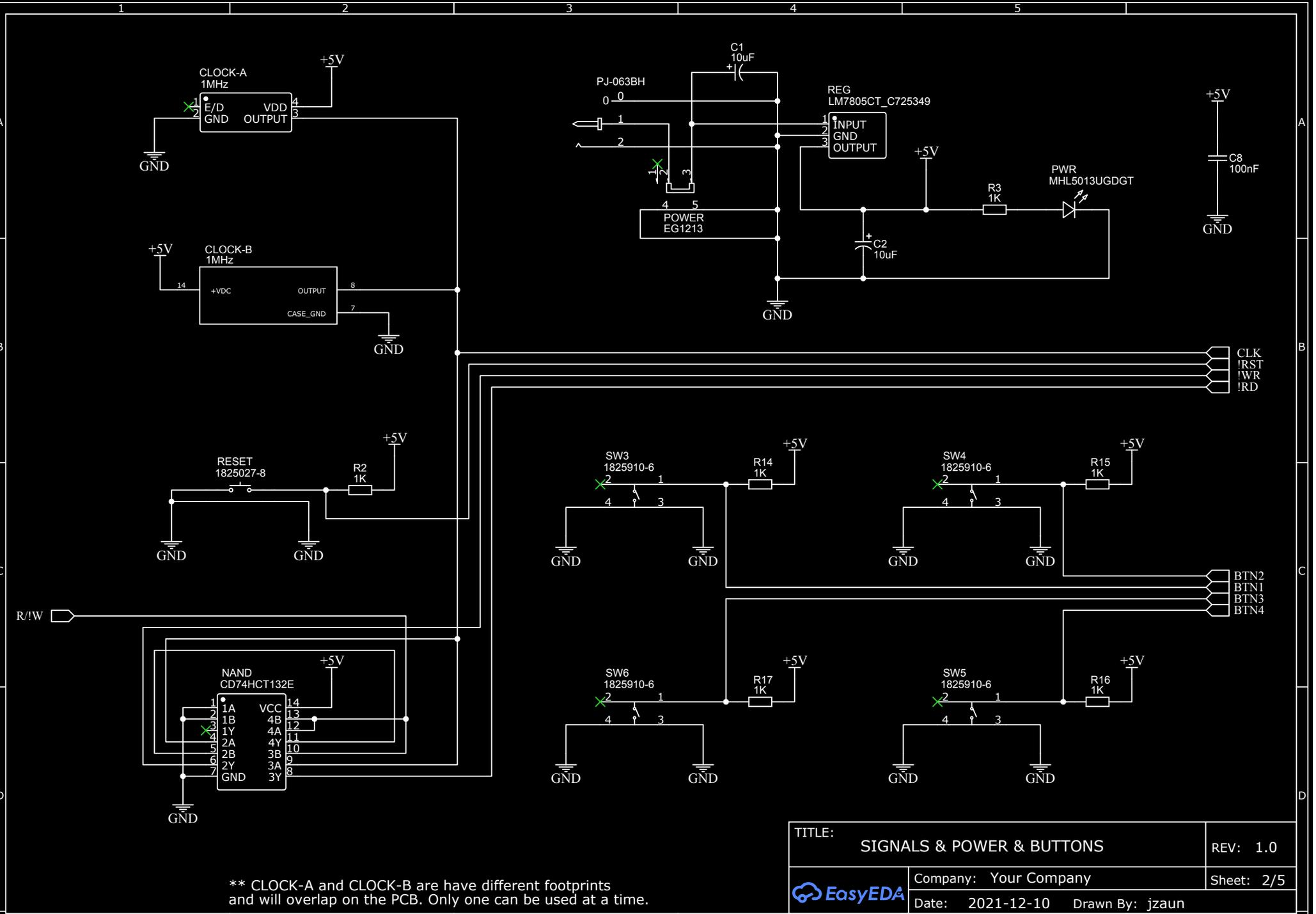
\*\* CLOCK-A and CLOCK-B are have different footprints and will overlap on the PCB. Only one can be used at a time.
